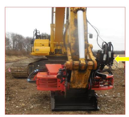
The stick pin will go to the top and the H-link pin will go to the bottom
