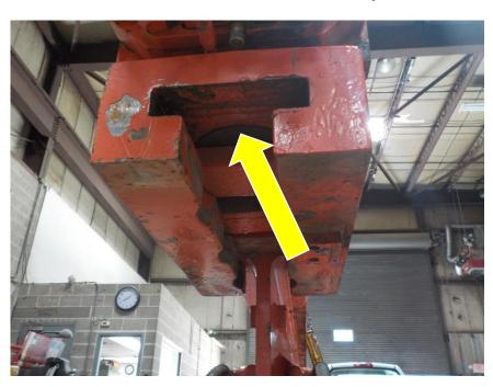
As you slide the clamp onto the beam all 3 wood blocks should slide out completely.
