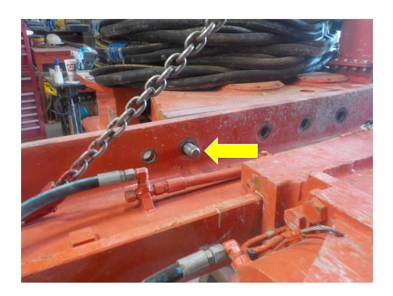
Apply a liberal coating of Anti-Seize Lubricant to the  $1 \frac{1}{2} \times 6 \times 4$  bolts. You will only need to apply it to the first 2 inches of threads.
