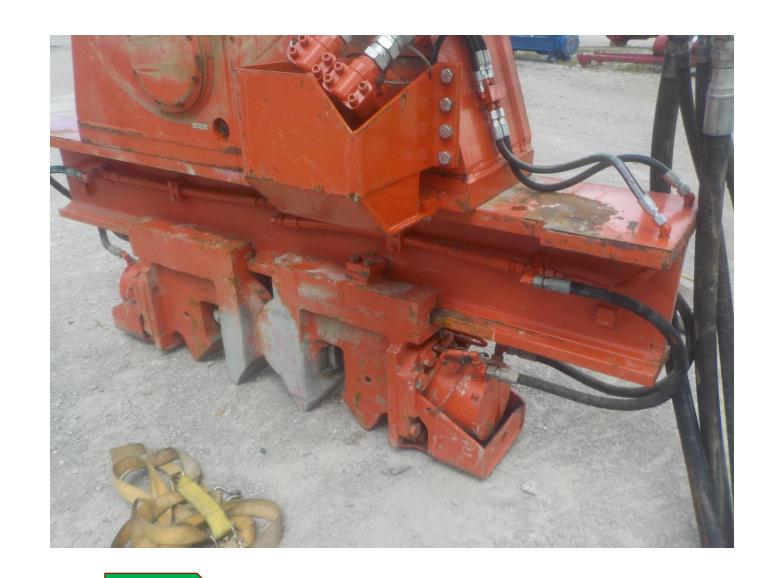
Open the check valve on the clamp cylinder. This will allow oil to be released from the cylinders that hold the clamps in place on the beam.
