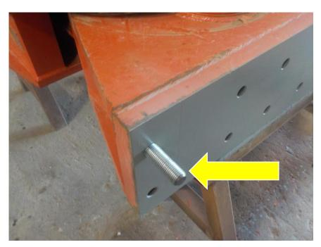
Make sure the bottom of the MKT V-22 is clean before mounting to the Beam
