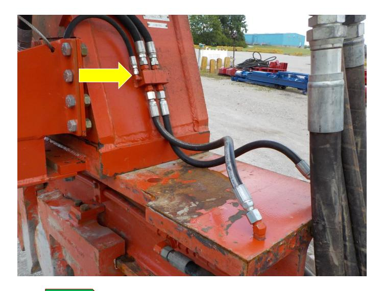
When ever the hydraulic lines of the MKT V-22 system have been reconnected and or when hydraulic repairs have been made, the clamp cylinders must be bled of entrained air.
