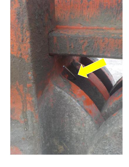
when ever the hydraulic lines of the MKT V-22 system have been reconnected and or when hydraulic repairs have been made, the clamp cylinders must be bled of entrained air.
