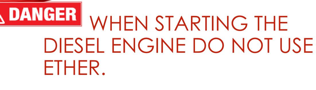
The engine is equipped with an electric heater starting aid and the use of ether may cause severe injury.
